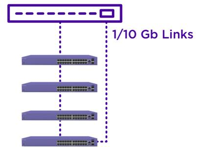
Cascaded V300/V400 switches in a Ring
