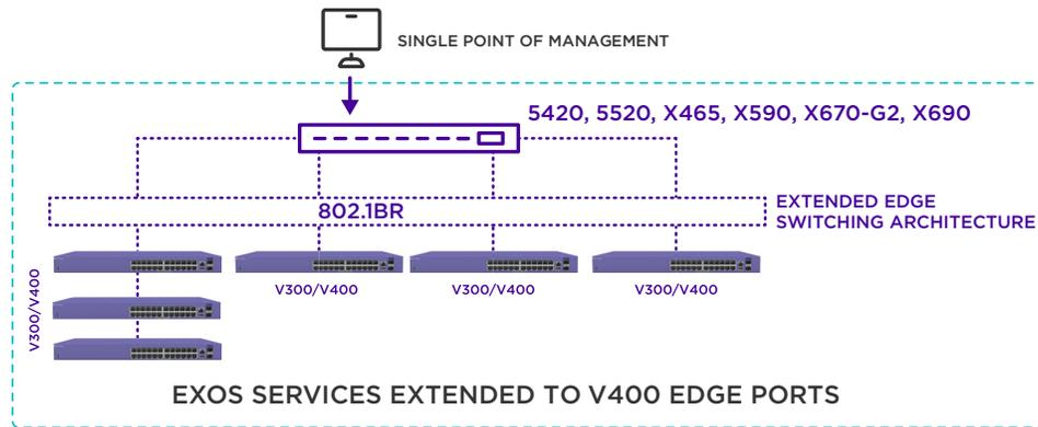
**Figure 1:** Extended Edge Switching extends aggregation switch features to V400 devices while providing a single point of management.
