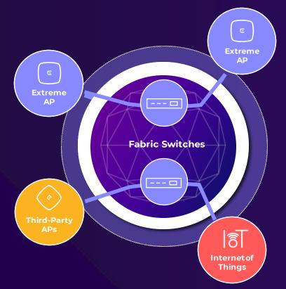
Fabric Attach extends the value of Fabric Connect to Extreme wireless access points, non-Extreme devices, and roaming wireless users. This increases network agility and better enables network architecture to scale business transformation initiatives sustainably.
