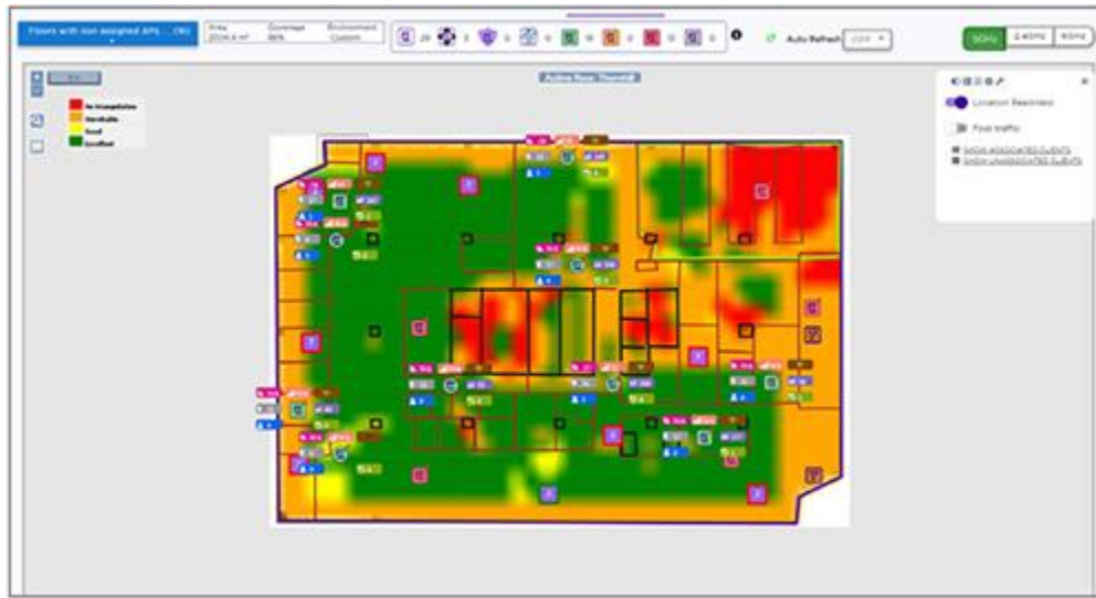
Figure 1: ExtremeCloud IQ Controller Wi-Fi Location Assessment
