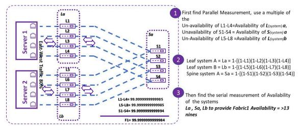
Figure 2: Availability Calculation of 3-stage Clos PoD Architecture based upon Extreme Networks SLX-series switches
