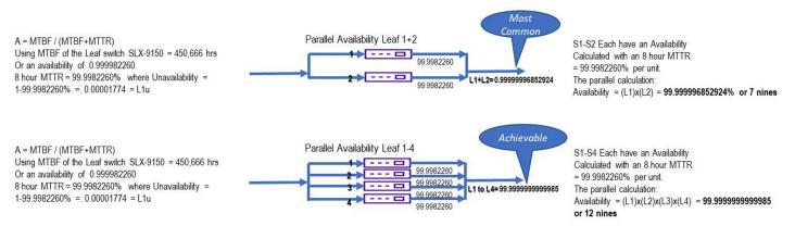
Figure 1: Availability Calculation of a parallel leaf-based system\* with 2 access ports to the Leaf, and 4 access ports to the leaf.
