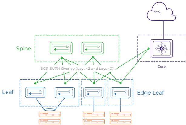
**Figure 1:** Extreme leverages BGP-EVPN and VXLAN open standards to enable controller-less network virtualization overlays to extend Layer 2 and Layer 3 reachability, ensuring easy and secure scalability.
