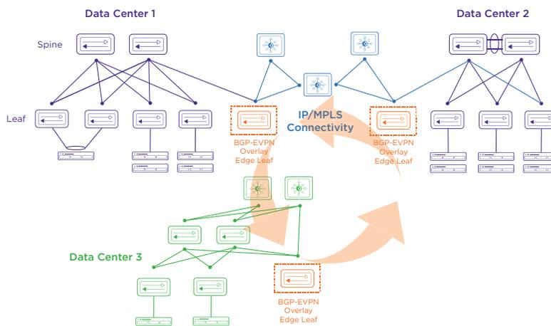
**Figure 2:** Extreme BGP-EVPN-enabled border leaf switches simplify DCI for Layer 2 and Layer 3 traffic.
