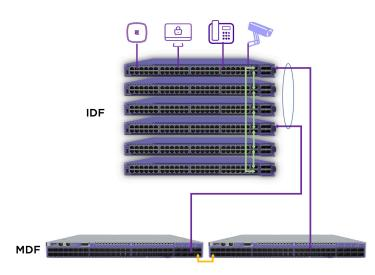
Within the IDF, switches are typically stacked providing a single point of management of all ports in the IDF reducing the number of elements to be managed in a network. User IP subnets typically span multiple IDFs, so it is very common to keep them as Layer 2 switches i.e. configure VLANs only on IDFs and provide default gateway routing functionality at the MDF layer.
