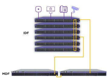
For infrastructure links such as uplinks as well as intra-IDF links, further reduction of edge configuration is achieved, by employing Zero-touch-fabric, which automatically establishes fabric connectivity among devices within an IDF, as well as towards the MDF, since there is no need to configure stacking or uplinks to the aggregation layer anymore.
