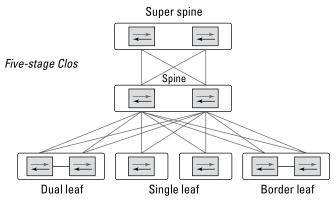
FIGURE 3-6: Three-stage and five-stage Clos designs.
