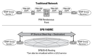
FIGURE 3-5: Multicast routing.
